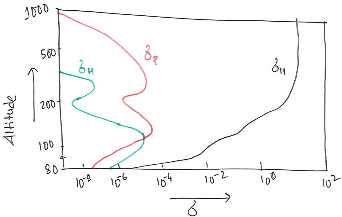
Since, the electron density  $\uparrow$  with altitude,  $\sigma_{||} \uparrow$  for  $\sigma_p$  and  $\sigma_H$ , they highly depend on  $\sigma$  which  $\downarrow$  as we move up in the atmosphere.
